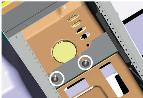
Utilize OEM flange nuts to finish the installation of Jotto Desk Contour Console, securing onto OEM mounting studs. This will snug up the console to the OEM dash.
